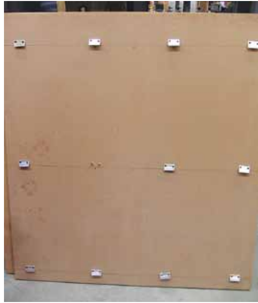
Figure 12: Test Set-up 3 - Panel Rear Side (Failed)
