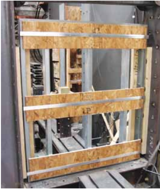
Figure 7: Test Set-up 2 - Wall Mount
